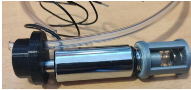
Figure 5 - Chemistry tube cap assembled with the solenoid and the plastic tube
