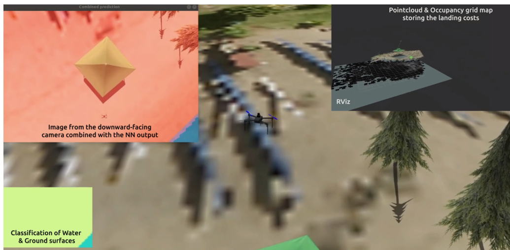
Figure 18: Overview of the Simulator Environment during the Landing process, along with the NN output (pure output and overlaid on the camera view) and the point-cloud from the stereo-camera overlaid onto the resulting cost map. The fitness of each position (cell) for landing is depicted through the grayscale value (black: unfit, white: fit for landing).
