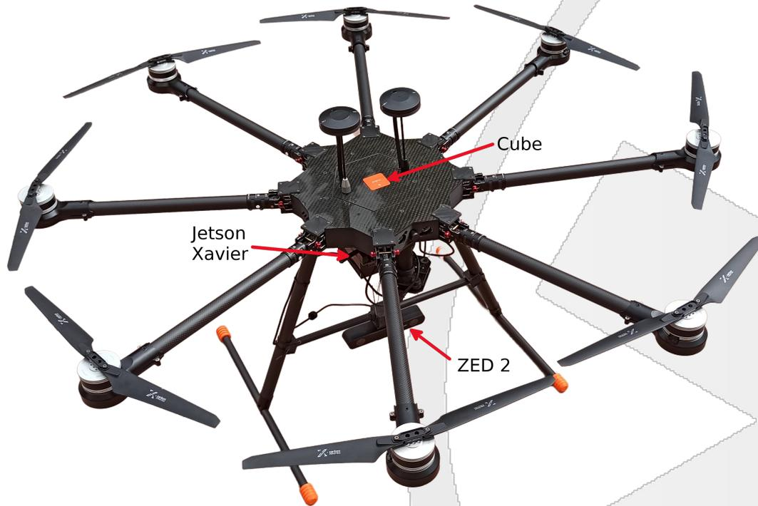
Figure 3: NTUA octorotor
